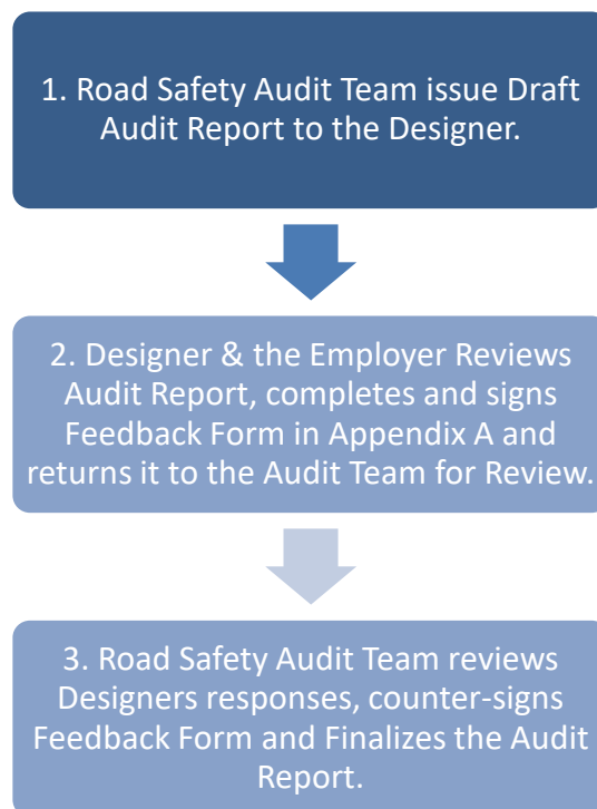
Figure 5.1 – Road Safety Audit Sign-Off and Completion Process
